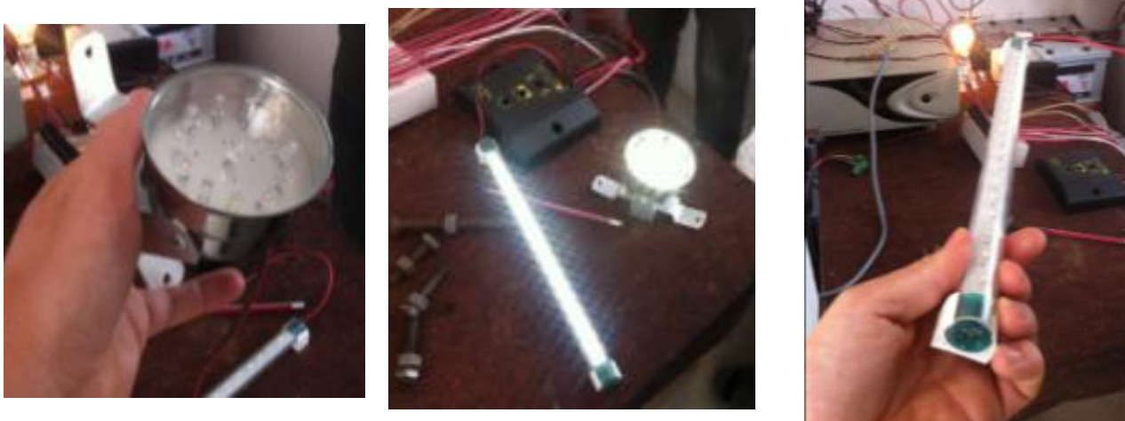
Figure 27: Lighting solutions developed and implemented by RIDS. Power demand 2,4 W (round), 1.8 W (longish).
